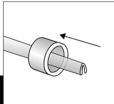
Fold hose to minimize width and slip a ProPEX ring over the end of the hose.
