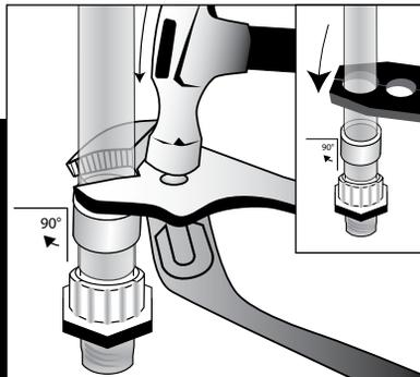
Drive ProPEX ring over fitting by holding pliers against ring at a 90° angle to the fitting and driving on with hammer, or drive on with PEX crimping tool. Allow room for fitting collar to turn.
